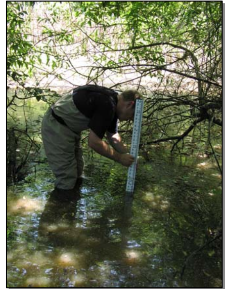
Installing a staff gage to measure surface water levels.
